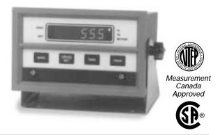
I he UMC555 is a rugged industrial digital weight indicator designed for simple operation in a variety of applications. The UMC555 is available in a mild steel painted enclosure with a tilt stand base, panel mounting brackets, or an uncased version for custom applications. Primary applications include platform scales, tank scales, truck scales, and railroad track scales.
