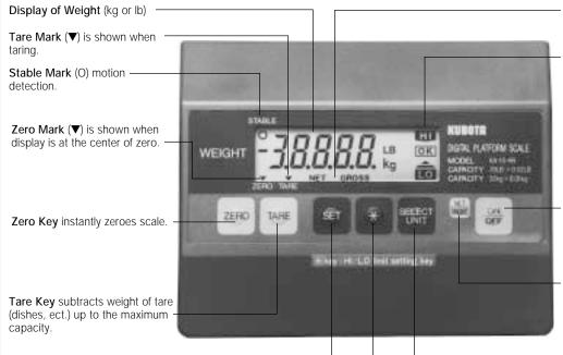
Set Key changes operating modes between over/under and straight weighing, or between counting and straight weighing (counting mode requires factory modification).
