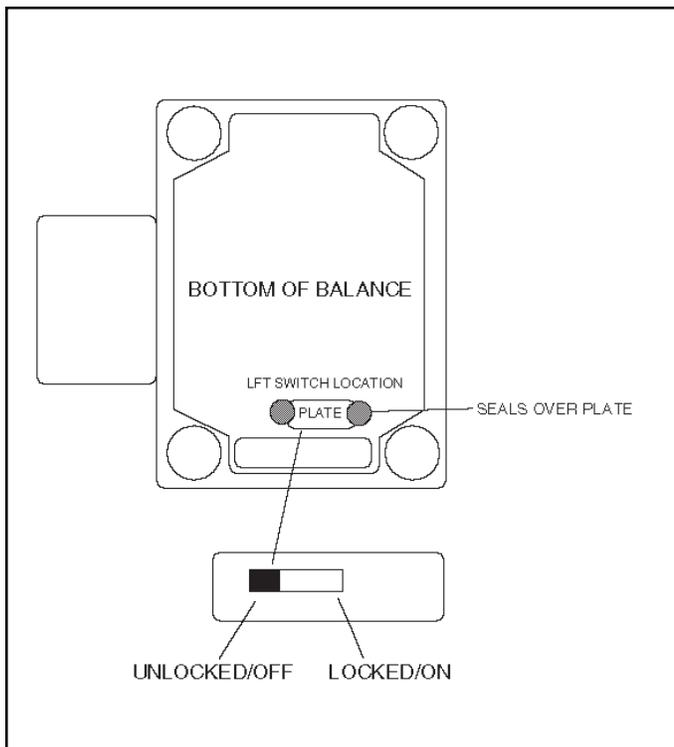
LFT Switch Location and Sealing Method
