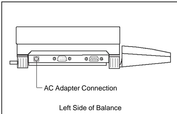
Connect the AC Adapter supplied to the three pin connector located at the left side of the balance.
