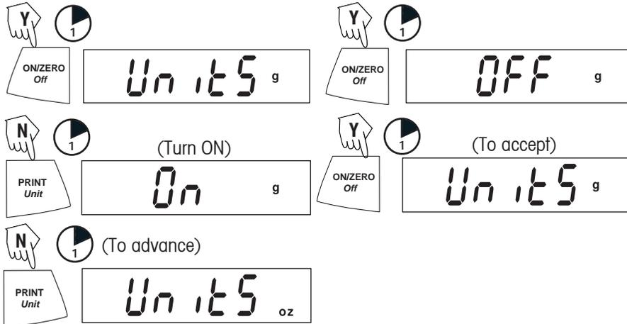
**NOTE:** Repeated presses of **PRINT Unit** button will go through all units, you then may select ON or OFF. Parts Counting is slightly different.
