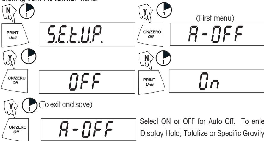
Select ON or OFF for Auto-Off. To enter Display Hold, Totalize or Specific Gravity, you must first enter the Mode sub-menu.
