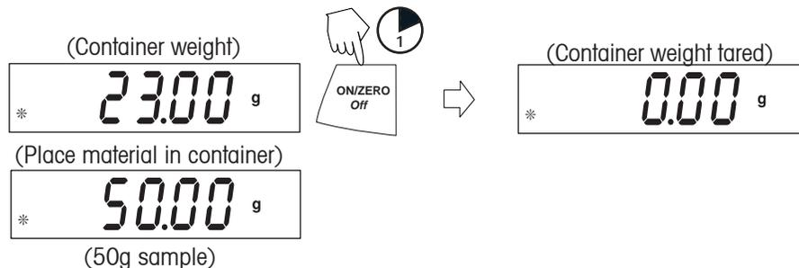
**NOTE:** Removing the container and material from the platform will cause the balance to display the container's weight as a negative number. The tared weight remains until **ON/ZERO Off** button is pressed again or the balance is turned off.
