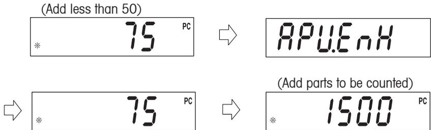
**NOTE:** The preceding procedure for enhanced counting can be repeated as many times as necessary providing the quantity added is less than the original entry.
