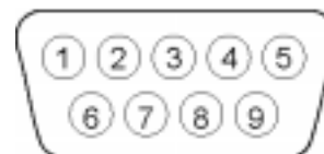
RS-232 Connector Pin Layout.
