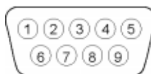
RS-232 Connector Pin Layout.
