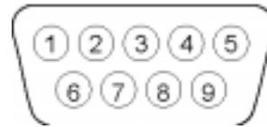
RS-232 Connector Pin Layout.
