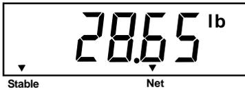
If enabled in program mode, additional units of measure may be utilized beyond the primary unit of measure used for callibration or display. Switching between primary and secondary units is accomplished by pressing the **Print/Units** button. Which unit is displayed depends on the current units being used. The following tables detail the graduation size conversions when switching between kg, lb and g.
