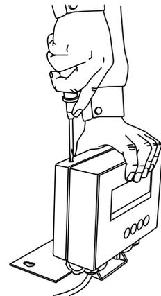
2. Insert the load cell cable through PG7 connector.
