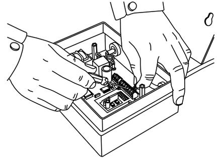
3. Connect the load cell cable to the main PCB according to the cable color code.
