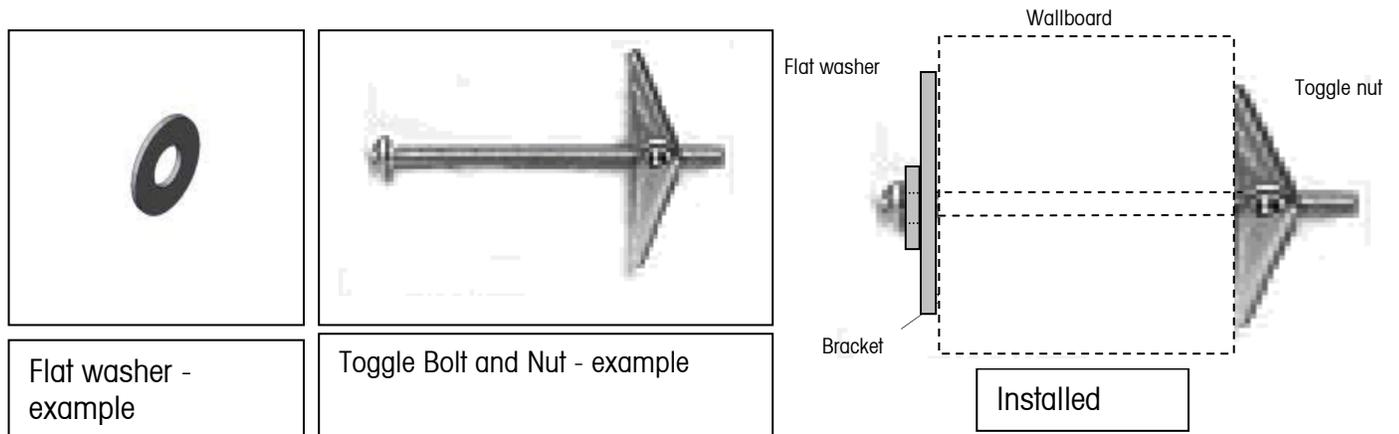
Recommended mounting bolt for wallboard and drywall: Type: Toggle Bolt, ¼" (6mm), minimum length 2-1/2" to 3" depending on wall thickness, pullout force of 900lb (450kg).
