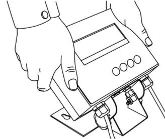
5. Place the XIF indicator on a desk or attach it to a wall with the optional wall-mount bracket. Plug the round connector from the power transformer into the side of the indicator. Plug the power transformer into a 120V AC outlet (indicator can also operate on batteries). To power up the indicator, press the On/Off (PRINT) key and hold it for three seconds.
