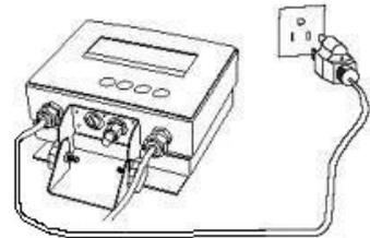
Check the scale to make sure that it is working properly. Place a known load or test weight equal to half the scale's rated capacity on the platform. If the recommended test weight is not available, use as much weight as possible to verify proper operation. If the scale indicator reads incorrectly, contact your authorized **METTLER TOLEDO Xpress** representative for help.
