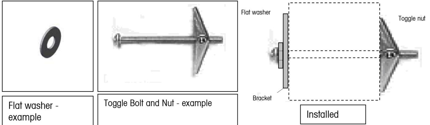
Recommended mounting bolt for wallboard and drywall: Type: Toggle Bolt,  $\frac{1}{4}$ " (6mm), minimum length 2-1/2" to 3" depending on wall thickness, pullout force of 900lb (450kg).
