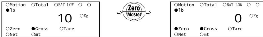
The scale will not accept a zero, or tare command, when the item being weighed is moving. The motion lamp lights to indicate that the item is in motion.
