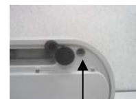
Transformer connection access hole
