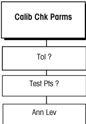
The Calibration Check Parameters sub-block enables you to specify the test parameters (default tolerance, number of test weight checks and alarm level) used in the calibration check procedure. The user will enter the number of test points and the starting value of the tolerance permitted between the test weight and the weight displayed on the scale.
