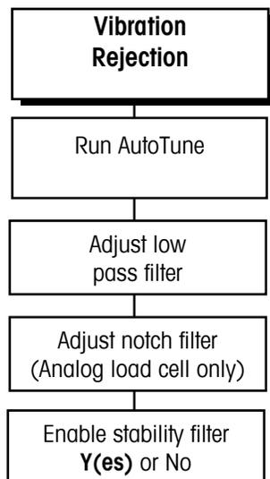
Note: Autotune is available only with analog load cell scale I/P PCBs of the revisions (or higher) listed below:
