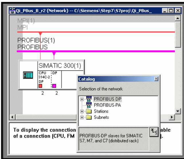
2.) The Qi Matroller is then dragged onto the Profibus Network
