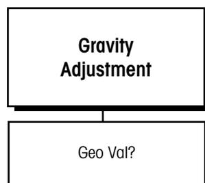
This sub-block allows you to enter a factor to compensate for gravitational differences between the factory calibration location and where the scale is currently located. If on-site calibration has already been performed, leave this value set to the factory default. When you access the **Gravity Adjust** sub-block, the current value is displayed.
