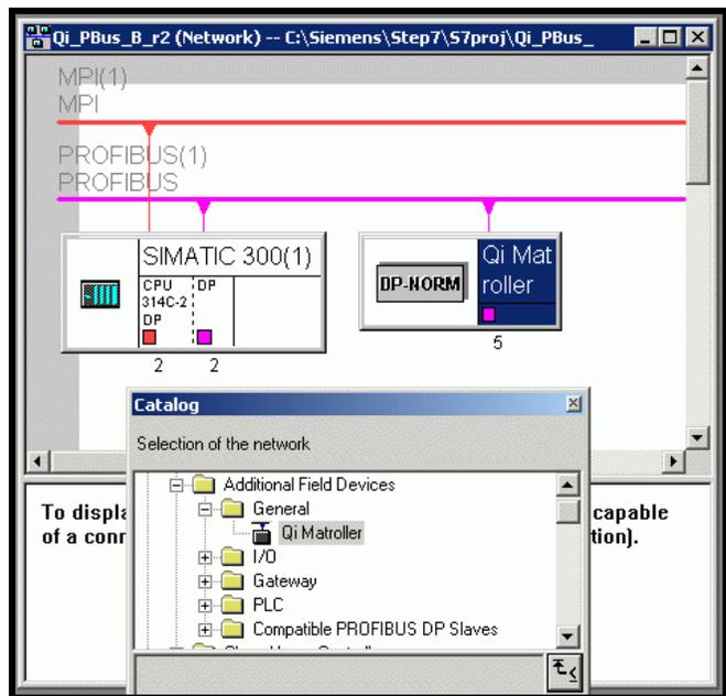
Step two is to configure the hardware. This means defining the I/O address locations.
