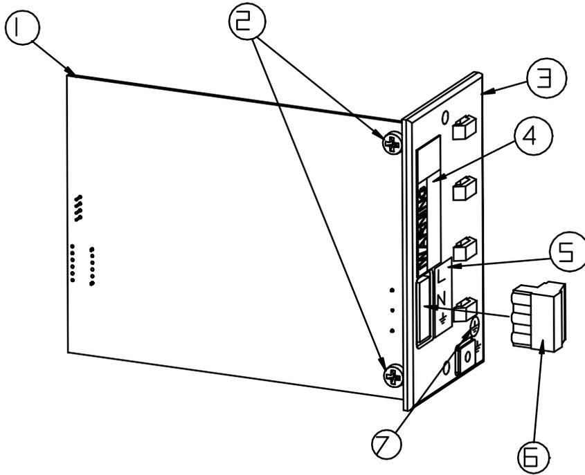
Figure 7f: Power Supply Assembly
