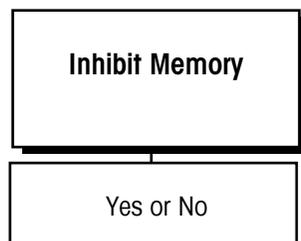
The Inhibit Memory sub-block is used to disable the MEMORY key on the Q.iMPACT matroller keypad. If **Y(es)** is selected, the MEMORY key will be disabled. If **N(o)** is selected, the key will function as normal.
