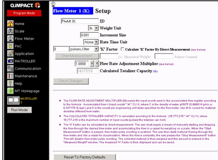
Fill in the weight unit, increment size, rate time unit, "K" factor, and the flow rate adjustment multiplier.
