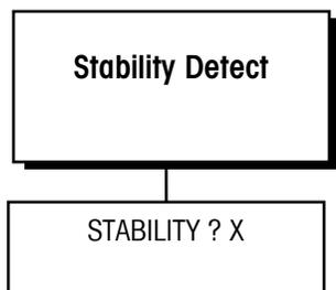
Stability Detection of a High Precision base is determined by the base electronics. The stability detection feature determines when a no-motion condition exists on the weighing platform. The sensitivity level determines what is considered stable. Printing and tare operations will wait for scale stability before carrying out the command.
