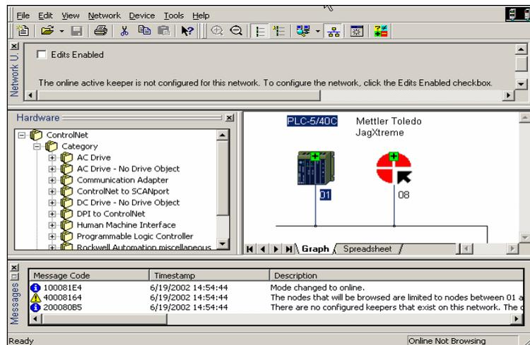
**Step 5** Check "edits enabled". With the PLC5 icon in focus select Scanlist Configuration from the Device pulldown menu.
