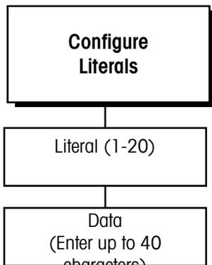
Literals are text strings, such as site name or address, that can be printed in a template. They can be up to 40 characters in length and are referenced by a field code (see the Configure Template Sub-block in this chapter). You can program up to 20 literals.
