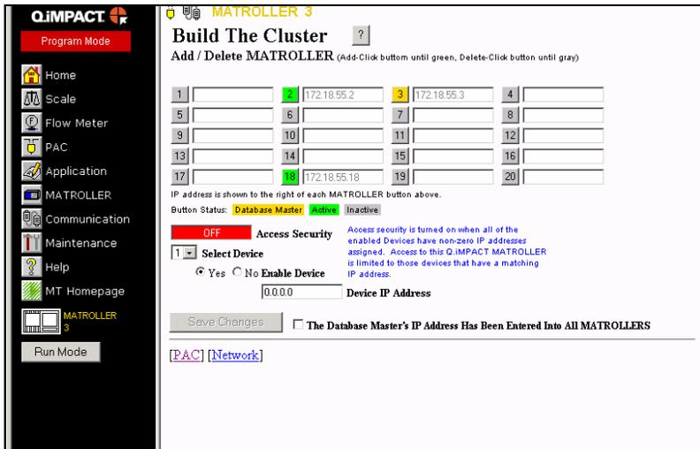
**!NOTE: All Matrollers in the Cluster MUST have a unique matroller number between 1 and 20. See Matroller section following**
