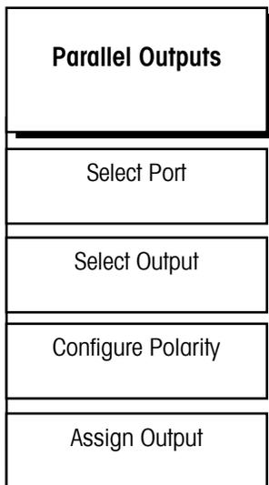
The Discrete Outputs sub-block lets you configure each of the four discrete outputs through PAR 2 (and an additional eight outputs for PAR 4 if an optional Multifunction PCB is installed). To configure outputs:
