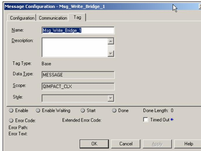
ControlLogix – screen shots showing configuration of the MSG instruction used to Read data to the Q.iMPACT matroller
