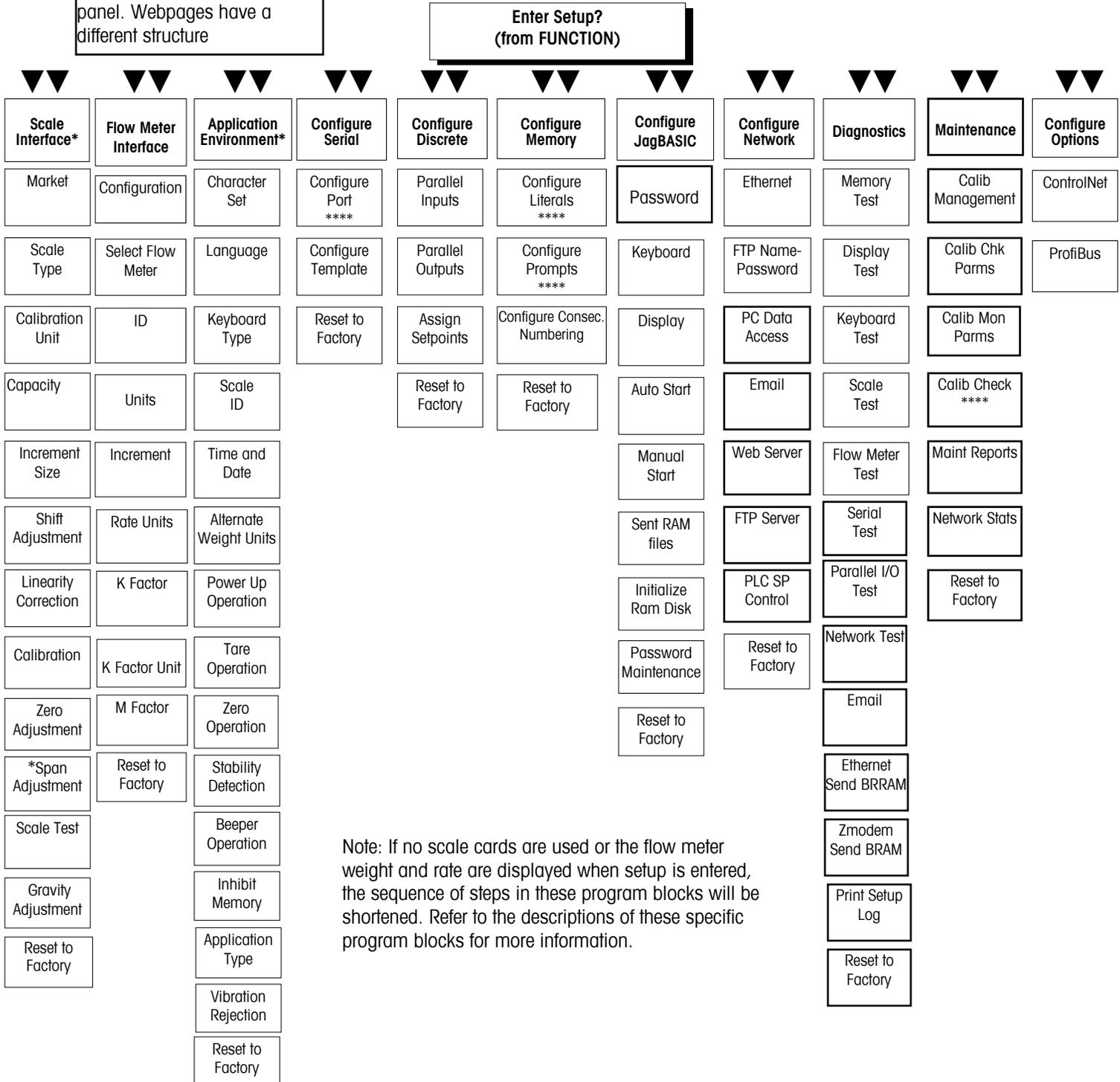
Note: If no scale cards are used or the flow meter weight and rate are displayed when setup is entered, the sequence of steps in these program blocks will be shortened. Refer to the descriptions of these specific program blocks for more information.
