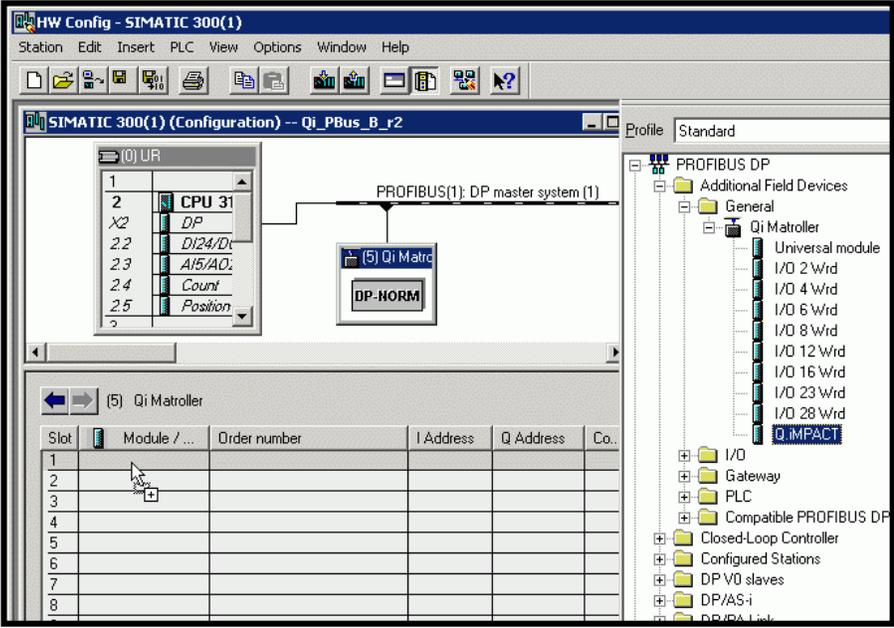
This shows the address mapping after adding the I/O mapping. In this example the Peripheral addressing starts at 256 for both Inputs and Outputs. The starting address's can be changed to suit your needs.
