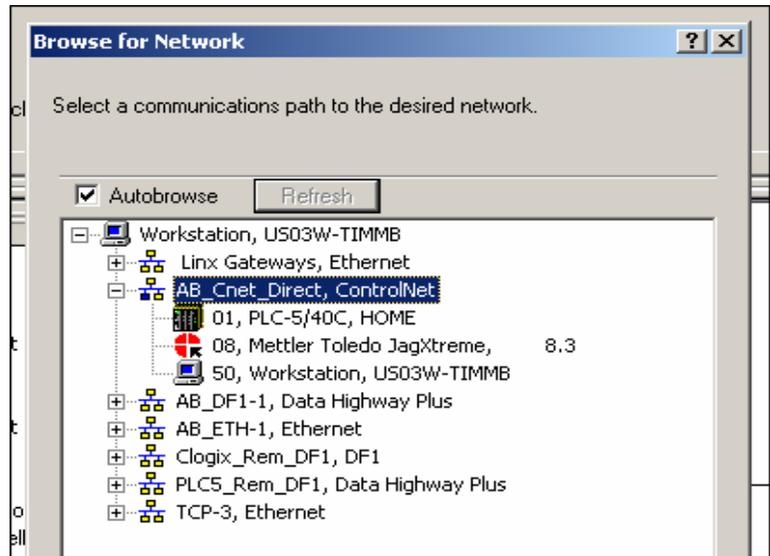
The screen below shows the result of the search. Results may vary depending on what type and how many devices are on the Network. Our example only has a single Q.iMPACT matroller with an address of 8.
