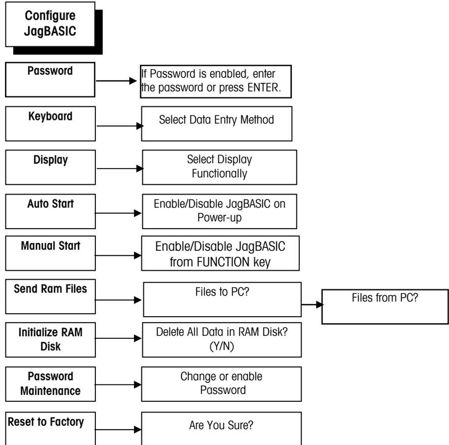
Enter the JagBASIC password to access the program block. If none has been entered since the last Master Reset, press ENTER to access the program block.
