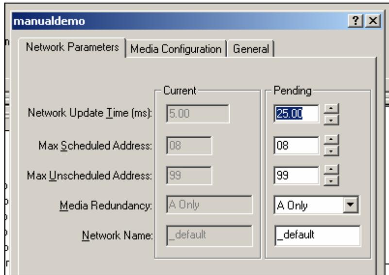
RSNetWorx will save configuration and update the keeper. Your Control Network is now ready for use with the Q.iMPACT matroller.
