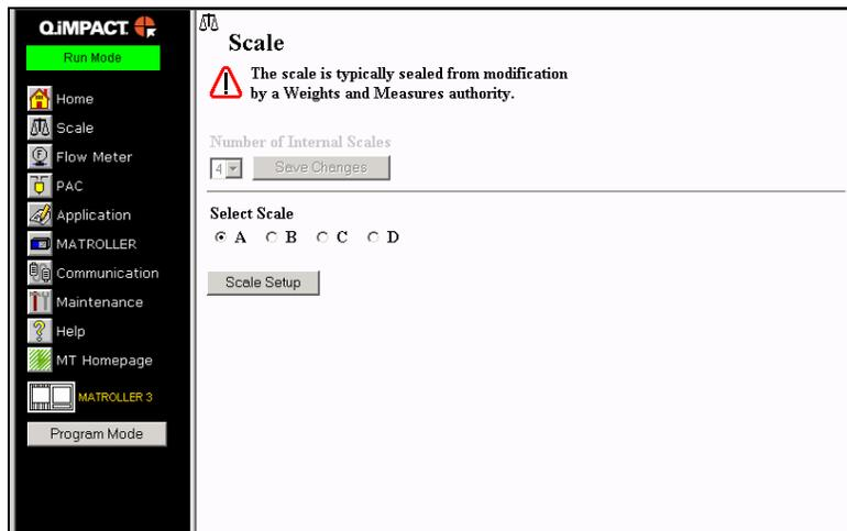
Clicking on the **Scale Setup** button takes you to the following screen. Set the parameters for the scale settings and adjustments. Click on **Save Changes** after setting up each step. A screen will appear with these symbols to denote that the step has been completed
