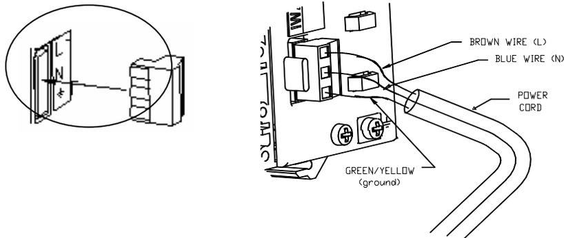
**Power Connections for Panel-Mount and Blind Panel-Mount Matrollers**
