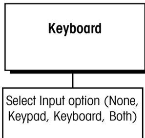
The Keyboard sub-block lets you select the type of device that will be used to input data to JagBASIC at an input or inkey prompt. The selected device is also used for BASIC command line mode.
