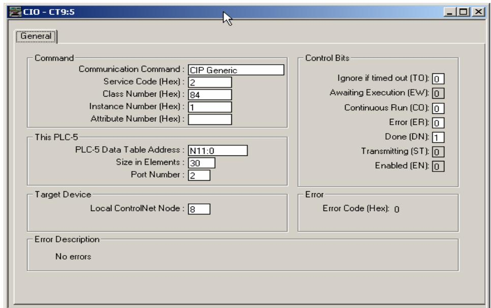
Example of PLC5 CIO write to Q.iMPACT matroller – class code 84h (note service code of 2).
