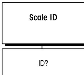
The Scale ID sub-block lets you assign an identification code to a scale for use in printing and when selecting a scale for operator viewing or interaction. The Scale ID can be up to 8 alphanumeric characters.
