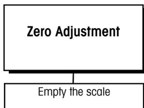
The zero value is the scale-empty reference as determined during calibration. The Zero Adjustment block lets you re-establish this value to compensate for any change since the last calibration. The scale must be empty before resetting the zero value.
