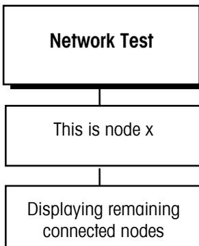
This sub-block tests the network connections. The test is done by first displaying the number of the local matroller, then requesting and receiving the node number and type of all other active nodes on the network.
