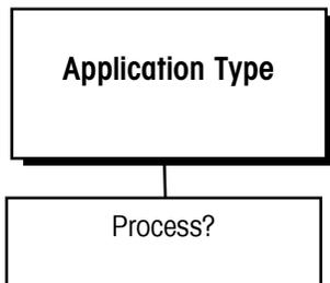
The Application Type sub-block indicates whether or not the scale is used for a process application. This sub-block affects the A/D rate and the ability to enable and/or disable the stability filter. To configure the sub-block:
