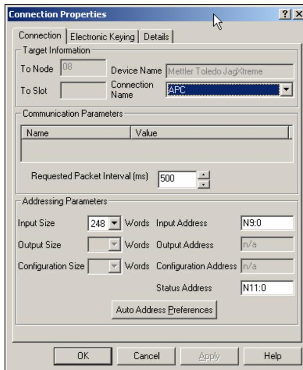
This window allows you to setup the cyclic data. First select the APC option from the "Connection Name" combo box. Then in the Input Address box enter the data file that the cyclic data should use. A recommended Requested Packet Interval would be between 250 and 500 ms. Assign the status data to the desired data file.
