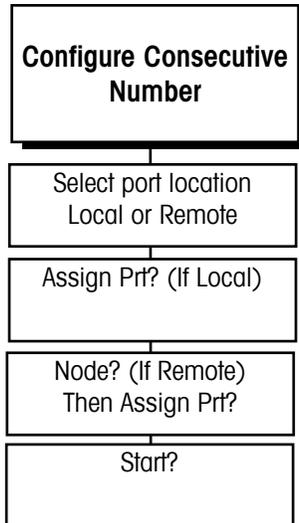
Consecutive numbering is used for sequencing purposes. The Q.iMPACT matroller automatically increments the number from a defined starting point.
