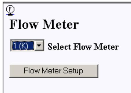
3. At first the screen, the parameters will be grayed out. You must switch the matroller to Program mode in order to continue. The screen below will then be displayed.
