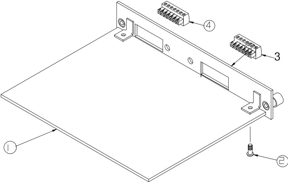
**Figure 7e: Dual Analog Load Cell PCB Assembly**
