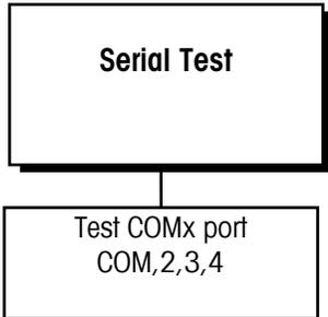
The Serial Test sub-block tests the serial I/O ports. You can transmit a test string of data to a designated port, or receive a string of input data. The input data scrolls across the lower display as received. You may see special characters representing control characters in the test string.
