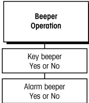
The Q.iMPACT matroller is capable of making an audible beep each time a key is pressed and an error alarm when an inappropriate key is pressed. This sub-block lets you enable or disable the keyboard sound.
