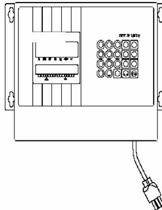
3. Tighten the brackets to the back of the enclosure (torque 25 inch pounds or 2.83 N•m).
