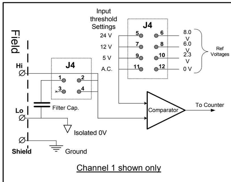
Schematic of Channel 1 Counter Input
