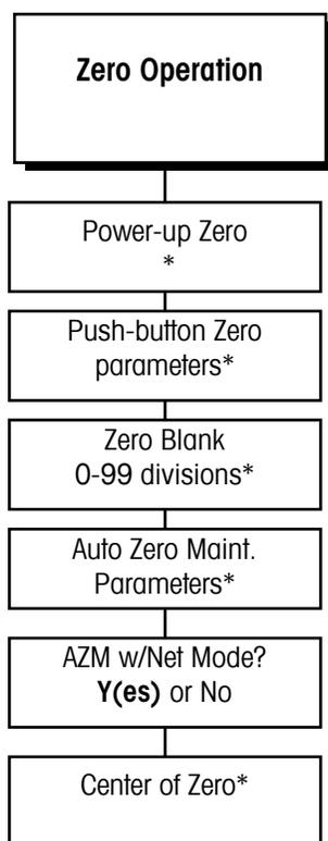
\*These menu selections are replaced by "Restart? Y/N" when Scale Type is High Precision (IDNET).
