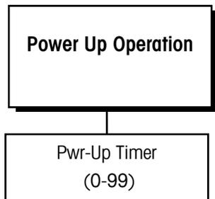
The Power Up Operation sub-block lets you specify a time delay before the scale is operational. This allows a sufficient warm-up period for stabilizing the scale and load cell electronics. The matrroller displays a countdown clock indicating the time remaining in the specified warm-up period.
