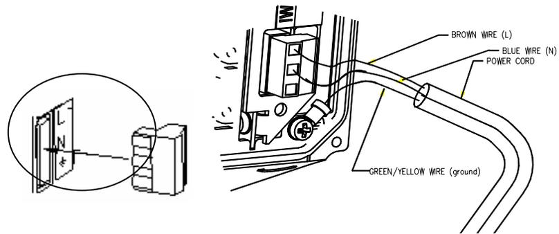
**Power Connection for Harsh Environment Q.iMPACT Matroller**
