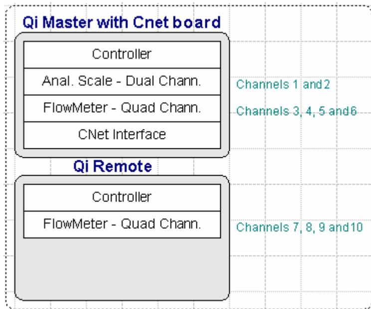
**Rear view of Q.iMPACT controllers showing placement of installed boards**
