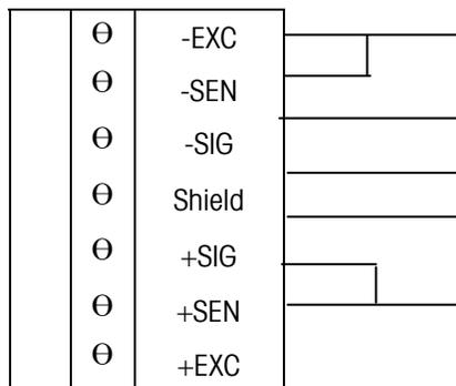
\* If an increase in load results in a decrease in weight display, reverse the signal wires (+SIG and -SIG).
