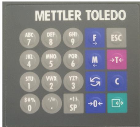
The keypad consists of a tactile-feel membrane switch covered with a polyester overlay. Audible beeps sound when a key is depressed.
