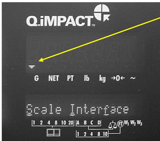
In the display shown here, the single arrow indicates you are in setup mode, top level.
