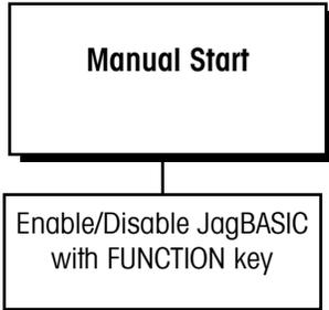
The Manual Start sub-block lets you configure JagBASIC as an operation associated with the FUNCTION key.
