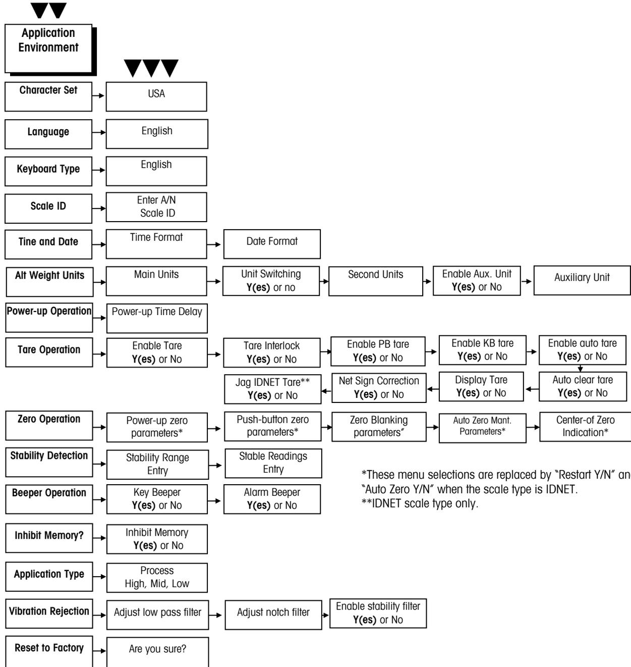
\*These menu selections are replaced by "Restart Y/N" and "Auto Zero Y/N" when the scale type is IDNET.
