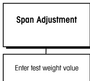
The Span Adjustment sub-block lets you make minor span adjustments without completely recalibrating the scale.
