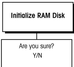
This sub-block lets you delete all files in the Q.iMPACT matroller's RAM disk and initialize it for new files.
