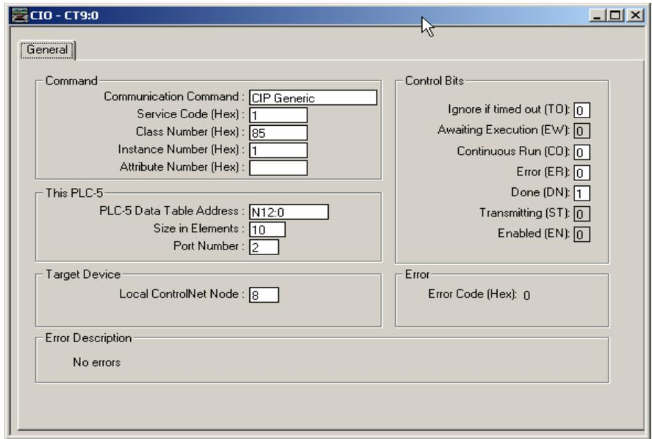
Example of PLC5 CIO read from Q.iMPACT matroller – class code 85 (note service code of 1)
