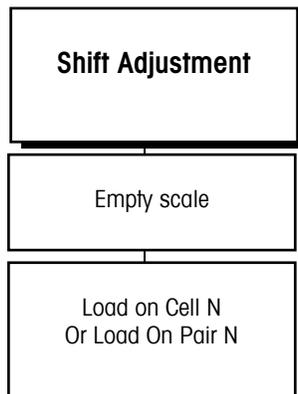
The Shift Adjustment sub-block lets you adjust multiple load cells connected to a POWERCELL (or RAAD box) scale. NOTE: It only appears if you selected POWERCELL in the Scale Type sub-block.
