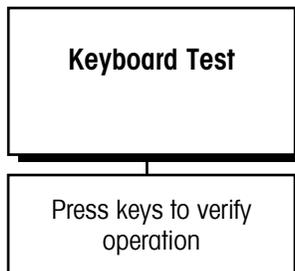
The keyboard test verifies the operation of each key on the Q.iMPACT matroller keypad or an externally connected PC/2 keyboard.
