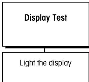
This sub-block tests the upper and lower display areas of the matroller and tests display ROM and RAM.
