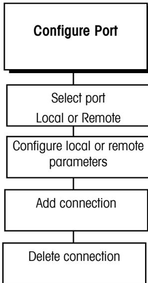
This sub-block lets you configure the serial ports on your local matroller for data exchange. You can configure only those ports that are physically available. For example, on a standard Q.iMPACT matroller with a single analog scale, you may have a remote display connected to COM 1 and a printer connected to COM 2.
