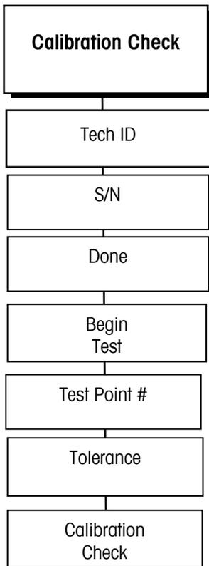
The Calibration Check sub-block section enables the user to perform the calibration test weight check with assistance from the Q.iMPACT matroller. The matroller will instruct the user through the test based on parameters entered in the Calibration Check Parameters section.
