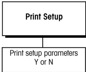
The Print Setup sub-block prints the matroller setup information as it is defined in the program blocks. It may be useful to have a hard copy of each matroller's setup parameters as back-up. Print setup data will be sent out the port that has been selected for demand output. If a network port has been selected, the data is sent through it.
