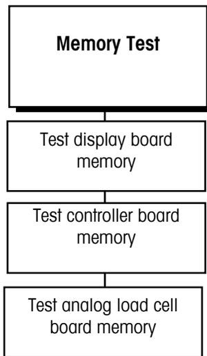
The Memory Test sub-block tests the matroller's internal memory. These diagnostics test the Flash memory, RAM, and EEPROM on the Controller board and any optional boards that are installed. The results of the memory tests are displayed on the matroller.
