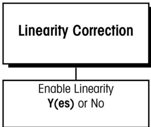
Linearity correction lets you calibrate the scale using reference weights at mid-scale and full-scale ranges. It allows for compensation of the non-linear performance of a load cell(s) or weighing system. If linearity correction is enabled, the calibration process requires additional steps. The matroller must be calibrated or recalibrated **after** you enable linearity correction.
