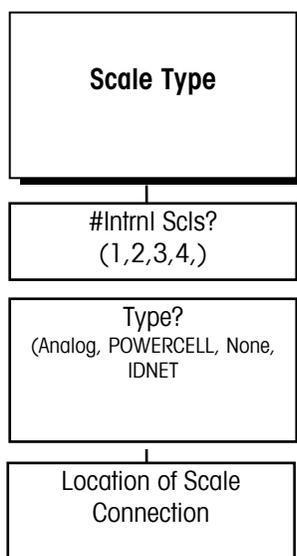
The Scale Type sub-block prompts you for the number of internal scales and type of scale that will be used.
