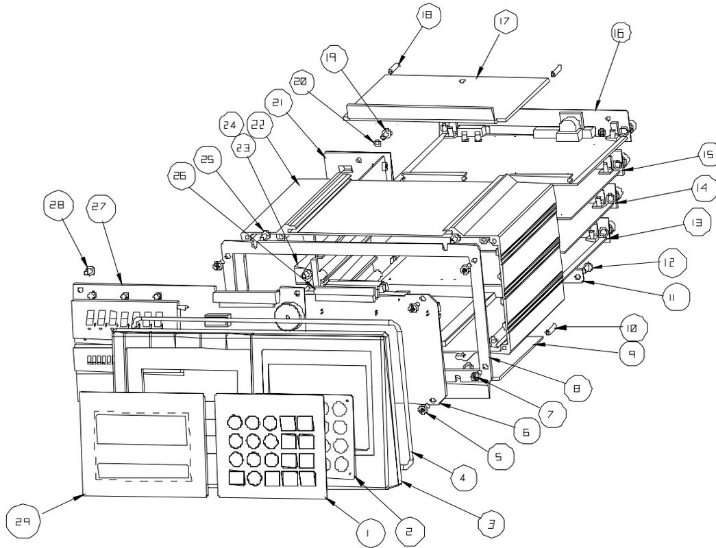
Figure 7-a: Panel Mount Model Parts
