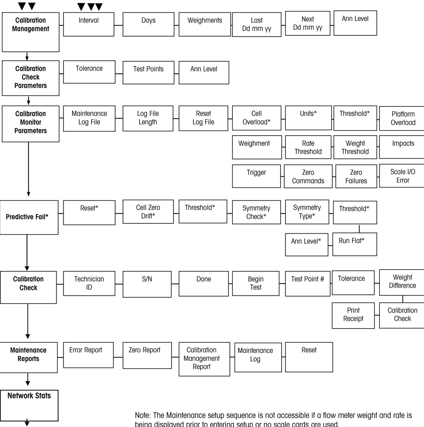
Note: The Maintenance setup sequence is not accessible if a flow meter weight and rate is being displayed prior to entering setup or no scale cards are used.
