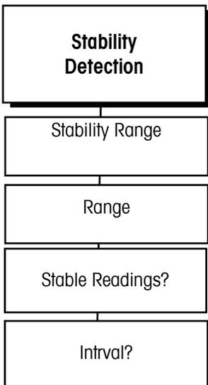
The stability detection feature determines when a no-motion condition exists on the scale. The sensitivity level determines what is considered stable. Printing and tare operations will wait for scale stability before carrying out a command.
