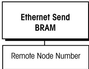
This sub-block allows you to send the Shared Data BRAM parameters from one matroller to another over the Ethernet LAN. You can setup the BRAM parameters on one matroller and duplicate them on another. Scale calibration parameters are NOT sent.
