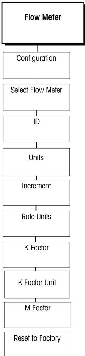
The Flow Meter Program Block is used to set the parameters for any flow meters connected to the system. (A flow meter option card must be installed.) At the Flow Meter Interface program block, press ENTER to access the block. At the Configuration sub-block, press ENTER. At the **[Select F.M.? 1]** prompt, choose the flow meter for which you are setting the parameters. At the **[ID? FlwMtr01]** prompt, the ID of the flow meter you are configuring will be displayed.
