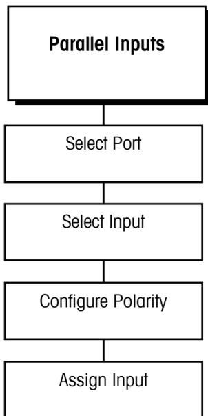
The Discrete Inputs sub-block lets you configure each of the four discrete inputs through PAR 1 (and an additional 8 on PAR 3 if an optional Multifunction PCB is installed). To configure inputs:
