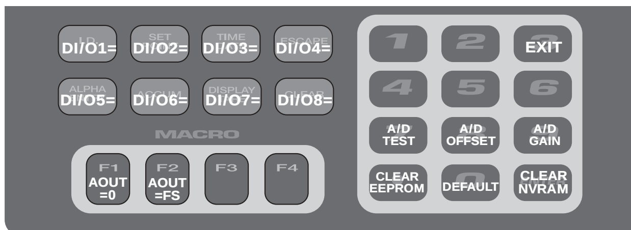
Figure 10-6. Front Panel Key Functions in Test Mode
