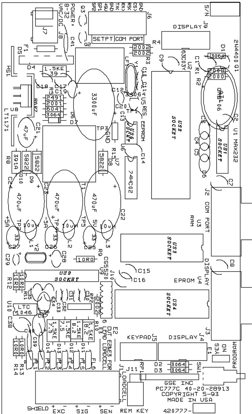
Figure 21-1 Main Board PC777C Component Layout
