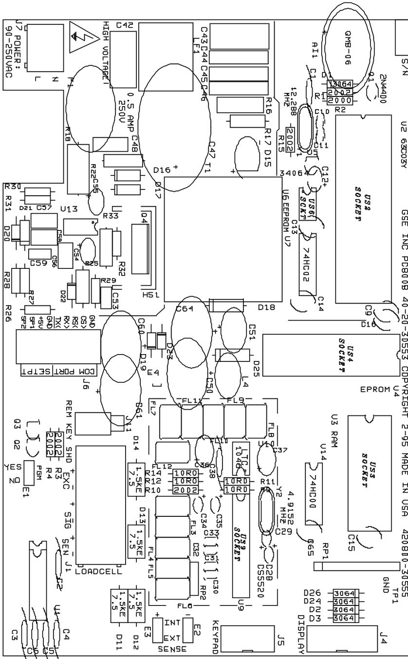
Figure 21-3 Main Board PC800B Component Layout
