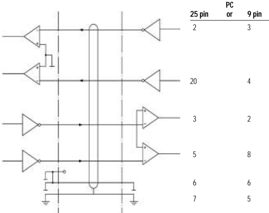
Type of cable: AWG 24 specification
