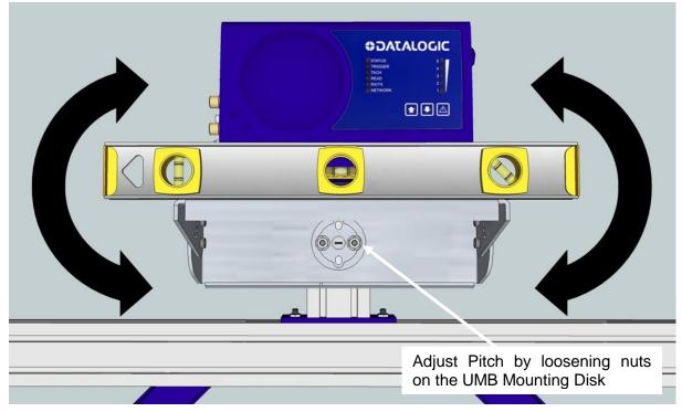
Figure 40: Adjusting the Pitch
