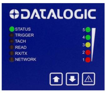
Figure 63: DM3610 Control Panel
