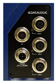
Figure 58: Connector Panel
