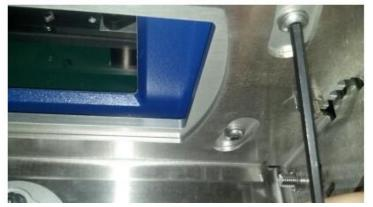
Figure 69: Removing a mounting bolt
