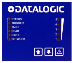
Figure 66: DM3610 Control Panel
