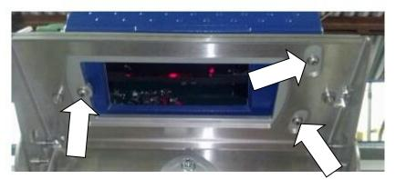
Figure 5.9: Mounting bolt location
