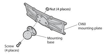
2 Now secure the assembly created in Step 1 to the back of the CV60 using the eight 1/4-20 x 5/8" screws provided.
