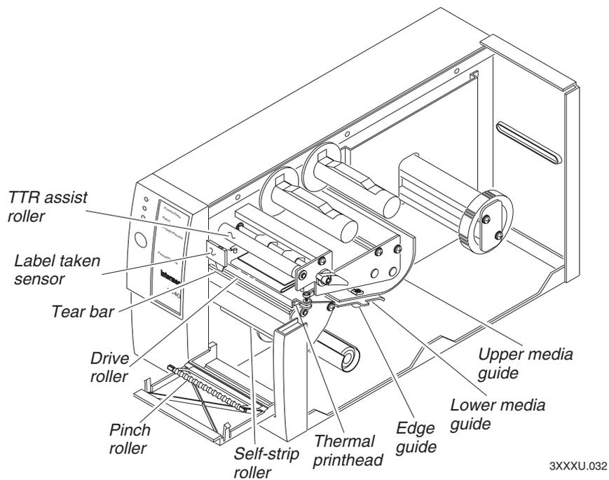
**Printer parts:** This illustration shows the printer parts that need to be cleaned. For a maintenance schedule of each part, see the Printer Maintenance Schedule table on pages 32-33.
