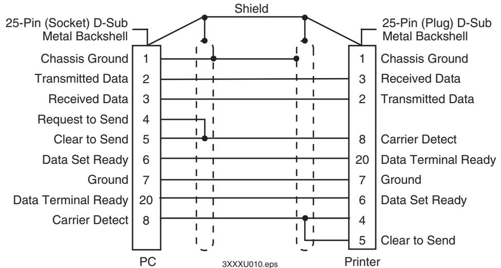
**RS-232 null modem cable for PC/XT:** This illustration shows the pin assignments for the RS-232 null modem cable for the PC/XT (P/N 048668).
