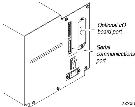
**Printer ports:** This illustration shows you where to connect your system to the printer.
