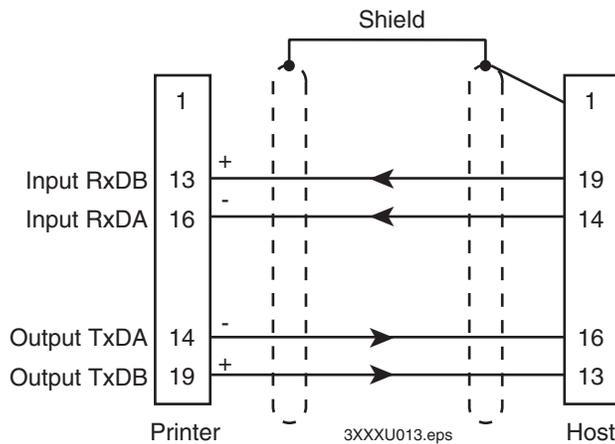
**RS-422 serial interface:** This illustration shows the pin assignments for the RS-422 serial interface. The host in this case includes Intermec products that support RS-422. Non-Intermec controllers may have different pin assignments.
