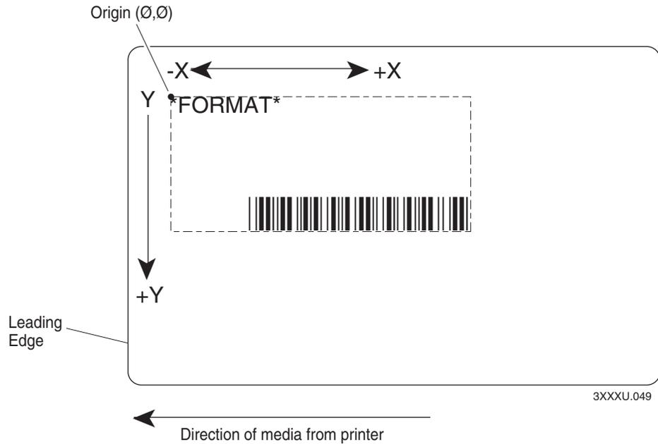
**Default X and Y origins:** This illustration shows the default X and Y origins. You can control the default X origin (top of form) with PrintSet or with the Test and Service DIP switches. You can control the default Y origin with the DIP switches only.
