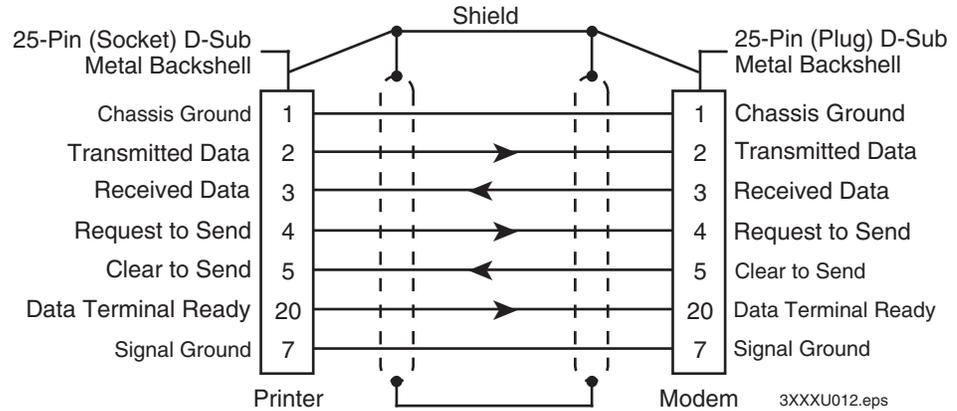
**Straight through DTE to DCE cable:** This illustration shows the pin assignments for the straight through DTE to DCE cable used with a modem (P/N 043237S). If you find that you are losing data, you may need to isolate the chassis ground from one of the two devices by connecting it to the shield.
