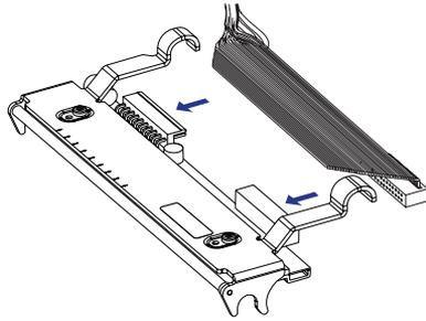
Connect the two cables to the replacement printhead.
