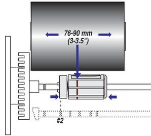
In case of 76 to 90 mm (3 to 3.5 inches) ribbon width, compress the ribbon supply bobbin and move it so it snaps into the second groove.
