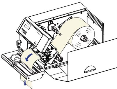
Route the media through the cutter between the two guide plates.
