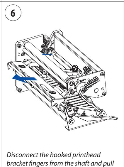
Disconnect the hooked printhead bracket fingers from the shaft and pull out the printhead as far as the cables allow.
