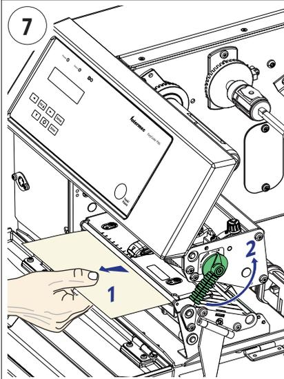
Pull out the cleaning card (1) and raise the printhead (2).
