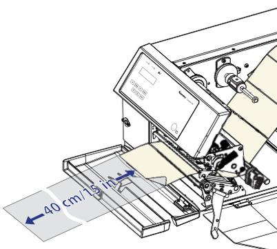
Pull out approximately 40 cm (15 in) of labels and remove the labels from the liner.
