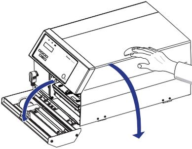
Switch off the power. Open the cutter and the side door.
