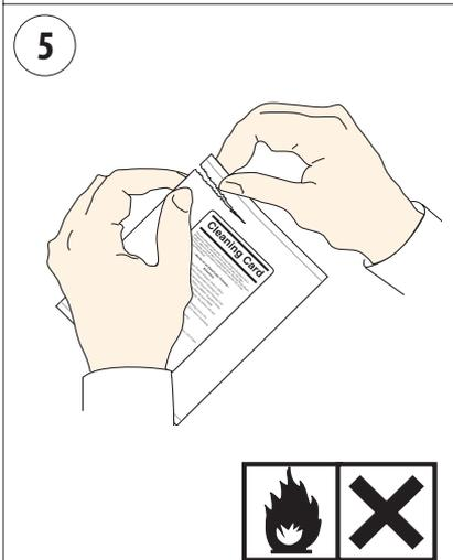
5 Open the cleaning card envelope and pull out the cleaning card. Read the warning text.
