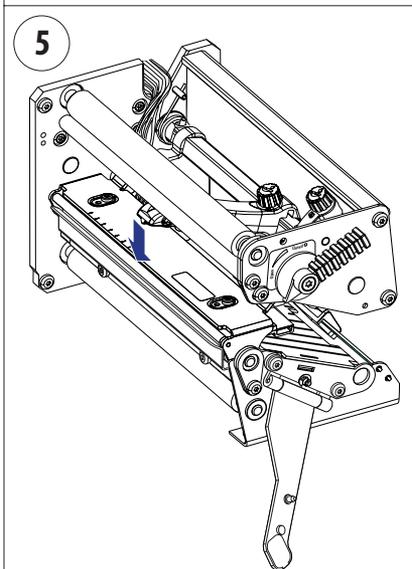
Pull the printhead bracket away from the magnet in the pressure arm.
