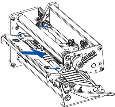
Fit the hooks of the printhead bracket fingers onto the headlift shaft. Make sure that the cables do not prevent the bracket fingers from being properly seated on the headlift shaft.
