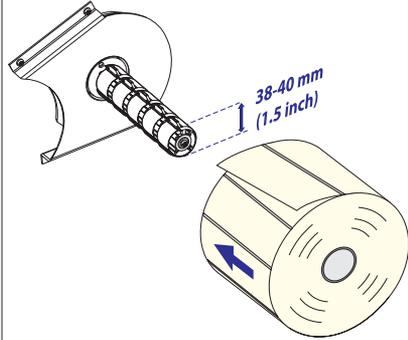
Fit a new roll of media on the media supply hub and push the roll inwards as far as it will go.
