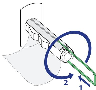
Secure the liner to the takeup hub with the clip (1) and rotate the hub (2) so the media becomes tight.
