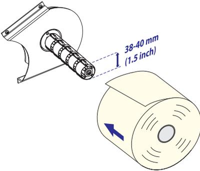
Fit a new roll of media on the media supply hub and push the roll inwards as far as it will go.
