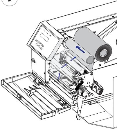
Press the cardboard core at the front end of the ribbon onto the rewind hub. During printing, the rewind hub will rotate counterclockwise.
