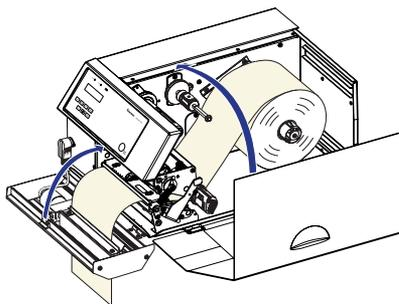
Close the cutter unit while pulling at the end of the media. Close the side door and switch on the power.
