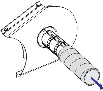
Remove any empty core from the media supply hub.
