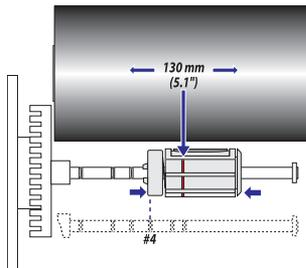
In case of 130 mm (5.1 inches) ribbon width, compress the ribbon supply bobbin and move it so it snaps into the fourth groove.
