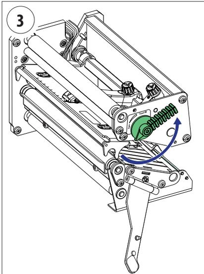
Turn the printhead lift lever counter-clockwise to raise the printhead.
