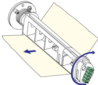
Route the media underneath the slack absorber and forward towards the print mechanism. The slack absorber can be rotated for better access and snap-locked in open position.
