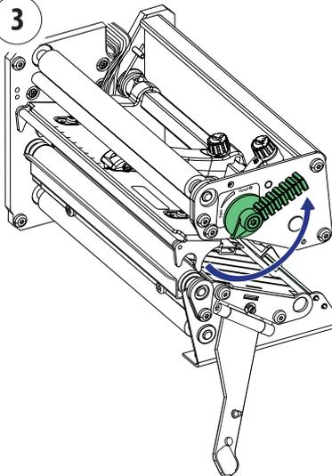
Turn the printhead lift lever counter-clockwise to raise the printhead.
