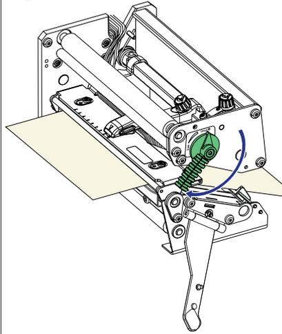
*Turn the printhead lift lever to "Closed" position.*
