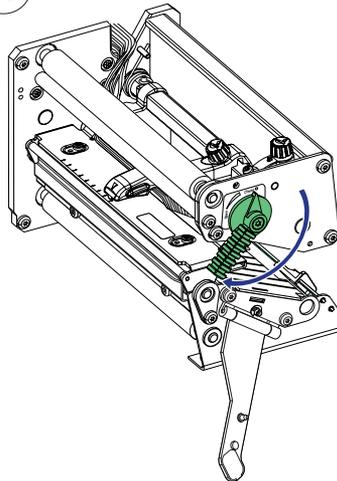
Close the printhead so the magnet engages the printhead bracket.
