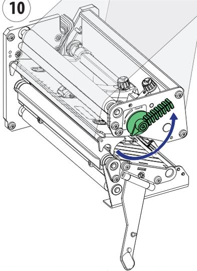
Turn the printhead lift lever to "Open" position.
