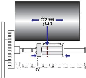
In case of 110 mm (4.3 inches) ribbon width, compress the ribbon supply bobbin and move it so it snaps into the third groove.
