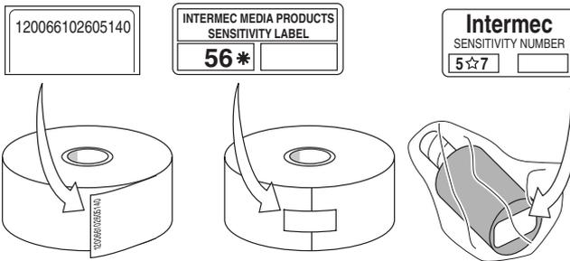
Use this three-digit number to optimize print quality and print speed on your printer. You can achieve the best print quality on the printer by using Intermec ribbon and media products.
