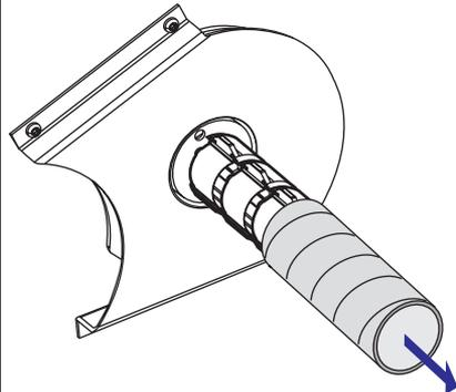
Remove any empty core from the media supply hub.
