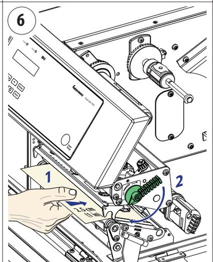
6 Insert most of the cleaning card under the printhead (1). Engage the printhead (2).
