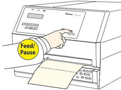
Press the Feed/Pause key to advance the media and adjust the media feed. Tear off the media by grabbing the outer edge and pull downwards.
