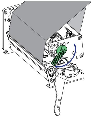
Turn the printhead lift lever to "Closed" position.
