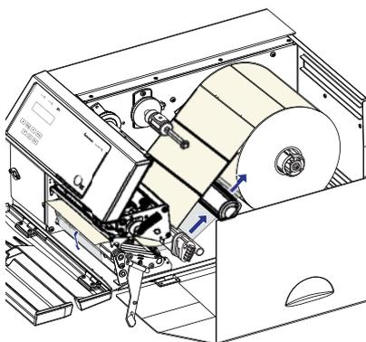
Route the liner around the tear bar and back under the print unit.
