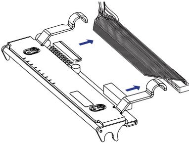
Disconnect the cables from the printhead. Note the snap-lock on the inner connector. Pull at the connectors—not at the cables!
