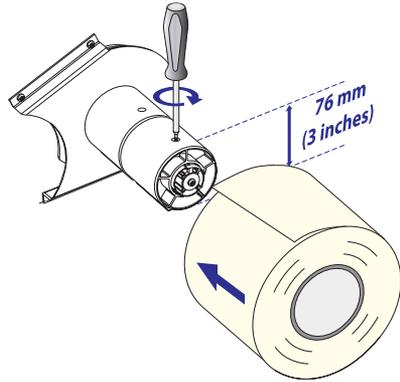
In case of a media roll with a 76 mm (3-inch) core, first fit two adapters on the media supply hub.
