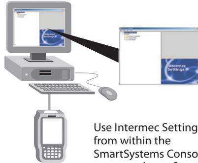
Use Intermec Settings from within the SmartSystems Console to remotely configure network parameters.
