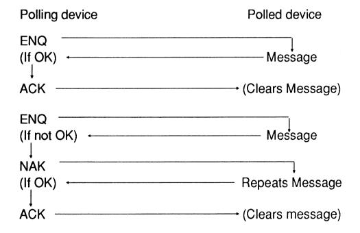
Note that ENQ/ACK/NAK can be replaced by user defined characters.
