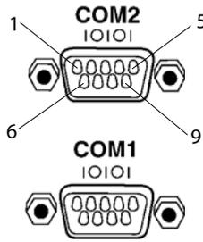
**COM Port Pinout (COM1 & COM2 identical)**
