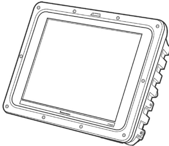
The CV60 display allows user input and menu navigation via resistive touchscreen. The touch panel is field replaceable.
