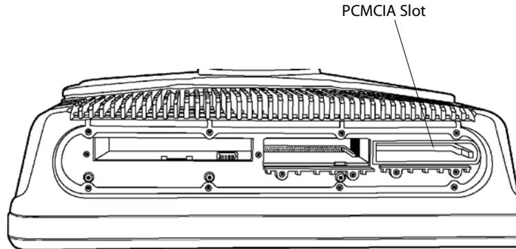
CV60 Top View (Radome Cover Removed)
