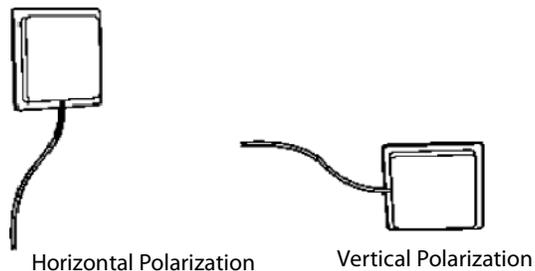
In mobile installations, best performance will be achieved by mounting the antenna flat, on top of the operator safety cage. Use at least two screws to hold the antenna in place.
