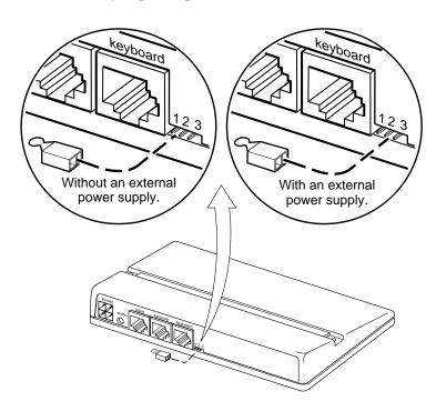
**Note:** Do not plug the power supply into the wall outlet until the reader is connected to the workstation and the keyboard, and you are ready to turn on the workstation.
