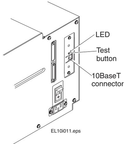
**Internal EasyLAN 10i2 Adapter:** This illustration shows the connector, LED, and button for the internal adapter.
