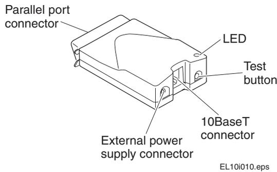
**External EasyLAN 10i2 Adapter:** This illustration shows the connectors, LED, and button for the external adapter.
