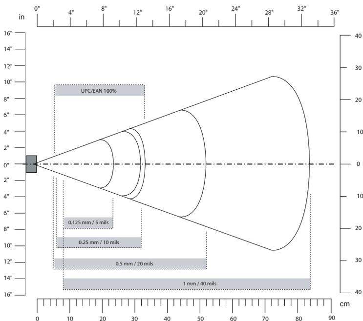
**EV12 Linear Imager Typical Reading Distances:** This graphic does not include the 1.5 mm (0.1 in) setback for the SR30.
