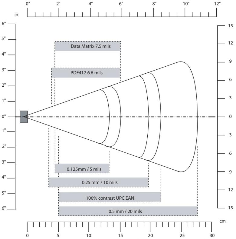
**EA15 Area Imager Typical Reading Distances:** This graphic does not include the 1.5 mm (0.1 in) setback for the SR30.
