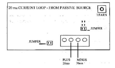
The AUTO-LEARN feature allows the unit to determine the Baud Rate and character format that is being sent to it. The unit will configure to the incomming data baud rate, data bits, and parity.
