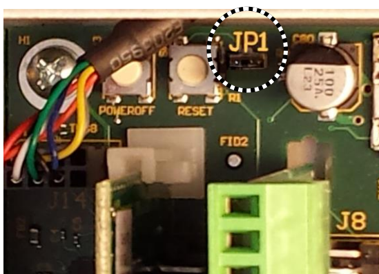
Installing the JP1 Jumper connection over both pins prevents accessing the Configuration and Service Menus from the front panel keypad
