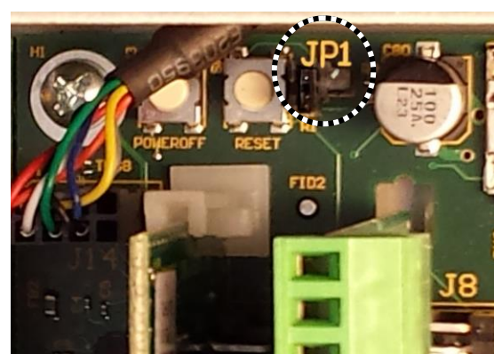
Disconnecting the JP1 Jumper and turning it side-ways allows access to the Configuration and Service Menu from the
