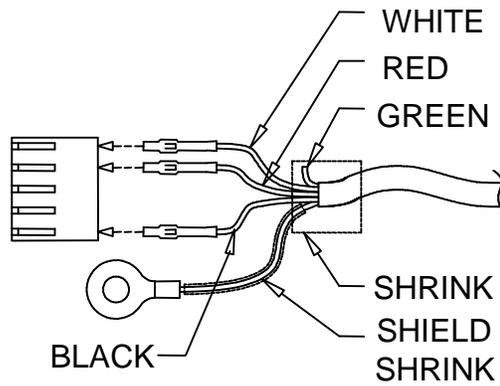
**Fig. 6: Connector J2, Serial cable assembly**
