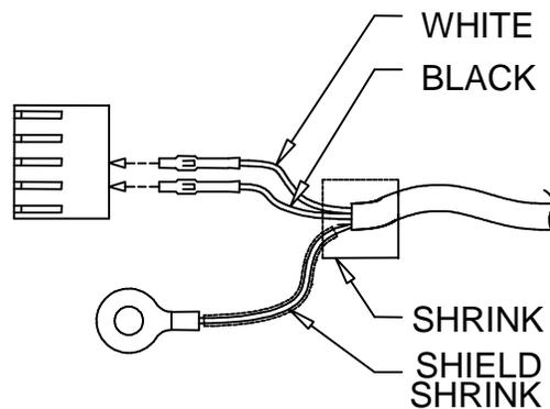
**Fig. 5: Connector J2, Remote switch cable assembly**
