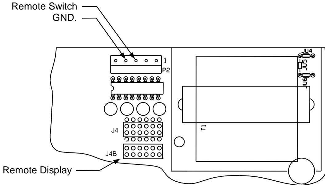
**Fig. 3: Remote Push Button Connections**
