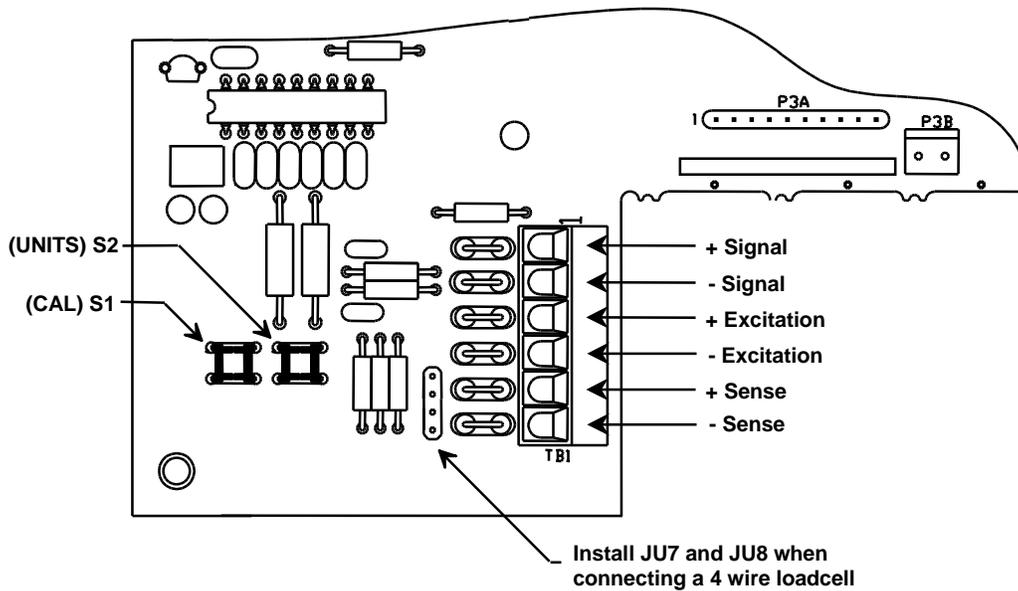
**Fig. 2: Load Cell connections**
