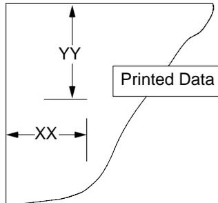
The general format for the input is  $A = YY.XX$  where  $A$  is the character identifying the data printed,  $YY$  is the number of lines down and  $XX$  is the number of spaces to the right.
