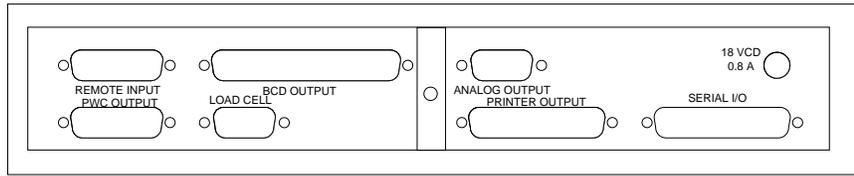
figure no. 2 - connector identification
