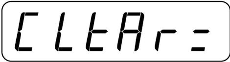
Press  to show the current setting. Press  or  to enter the new setting. Then press  to save it or to save the current setting. Clear tare on completion of the transaction (a negative net weight after display of a positive net weight).
