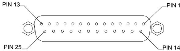
**Standard "Printer Connector RS-232C Pin Definitions:**
