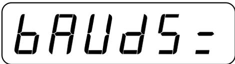
Press  to show the current baud rate. Use the numeric keys to enter a new baud rate for the bi-directional serial post. Then press  to save it or to save the current setting.
