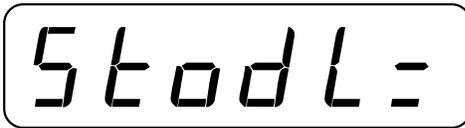
If "C" numbers were entered, remove all weight from the scale, press  then press  to display *YES*. Press  to store the current scale weight as the deadload
