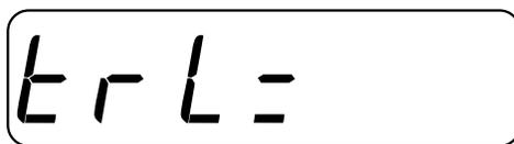
Press  to show the current setting. Press  or  to enter the new limit for zero range. Then press  to save it or to save the current setting.
