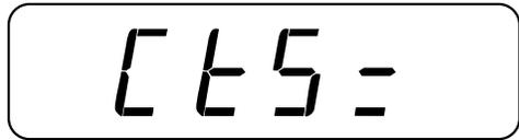
Press  to show the current setting. Press  to disable or  to enable the Clear to Send (Printer Output Handshake) for the printer output. This feature can be used with printers that have small buffers to prevent data overrun. Press  to save it or to save the current setting.
