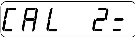
This is the second of two calibration weights. If the first weight (*CAL 1*) was zero, this weight should be equal to the test weight total. If, however, the first weight was the test weight total, then this weight should be zero. Press the  key. The display will show 0. If this second
