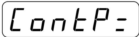
Press  to show the current setting. Press the  or  to enable or disable the continuous serial output on the printer serial port. A NO selection enables print switch operation. Then press  to save it or to save the current setting.
