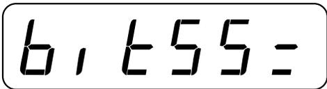
Press  to show the current number of data bits. Press  or  to enter the new number of data bits for the bi-directional serial port. Then press  to save it or to save the current setting.
