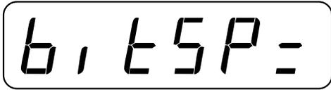
Press  to show the current number of data bits. Press  or  to enter the new number of data bits for the printer serial port. Then press  to save it or to save the current setting.
