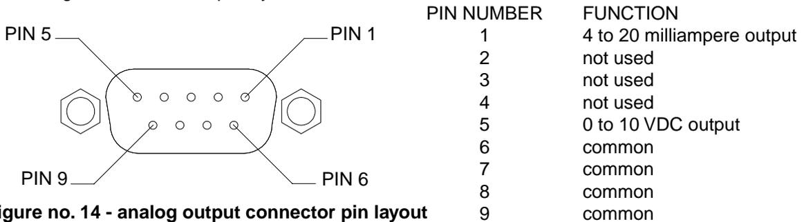
**figure no. 14 - analog output connector pin layout**
