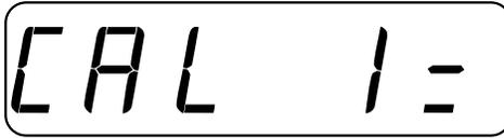
weight. This is the first of two calibration weights: NO LOAD or ZERO and the TEST WEIGHTS or TEST LOAD. Press the  key and the display will show  for NO LOAD. If the first calibration weight is to be ZERO or NO LOAD, press the
