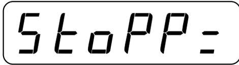
Press  to show the current number of stop bits. Press  or  to enter the new number of stop bits for the printer serial port. Then press  to save it or to save the current setting.
