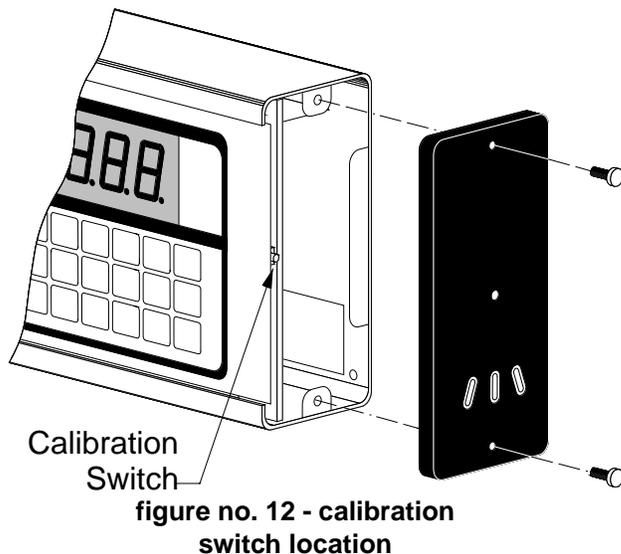
If you have a 748 desktop enclosure, it will be necessary to remove one of the end caps from the enclosure to gain access to the calibration switch. To do this, first remove the instrument from the gimbal mounting by removing the two (2) large knobs. Make certain that the smaller locking screw on one side is first loosened. Next, remove the top and bottom screws from the right end cap (see figure no. 12). The switch is located on the printed circuit board near the center.
