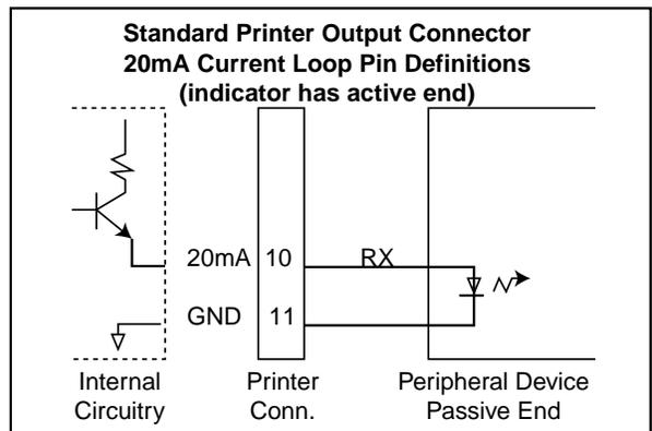
figure no. 4 - printer output connection
