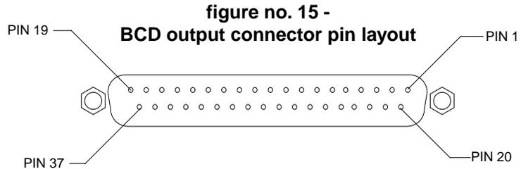
**figure no. 15 - BCD output connector pin layout**
