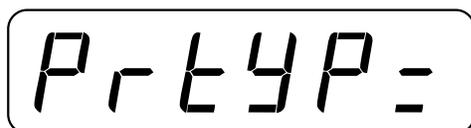
Press  to show the current parity setting. Press  through  to enter the new parity setting for the printer serial port. Then press  to save it or to save the current setting.
