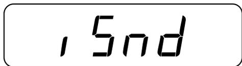
YES/NO to inhibit sending serial data during input. If yes, all serial output will stop while weight is not being displayed (i.e. while inputting id, tare, time, date, presets, bargraph or displaying the current tare value). **NOTE:** YES required for "Legal for Trade" applications.
