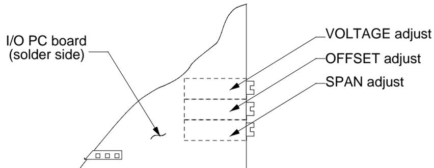
**figure no. 17 - analog output calibration adjustment**
