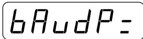
Press  to show the current baud rate. Use numeric keys to enter the new baud rate for the printer serial port. Then press  to save it or to save the current setting.
