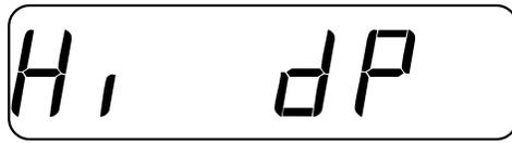
Press  to show the current setting. Press  through  to enter the desired decimal point location and press  to save it or to save the current setting. Must be the
