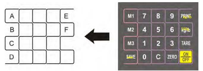
6. Press the "C" and the scale will show the version, count up, and then go to the weigh mode.
