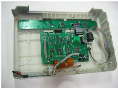
2. Remove support frame and replace main board.
