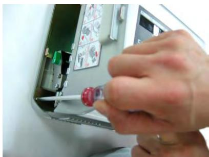
Remove front cover bolt (2 bolt)
