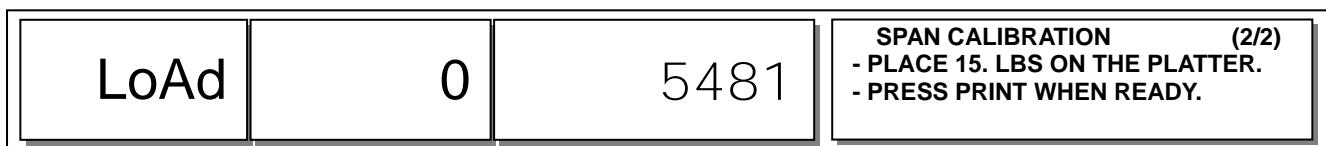
③ Place the maximum capacity on the platter. (Menu 8130 sets the max capacity for calibration.)
