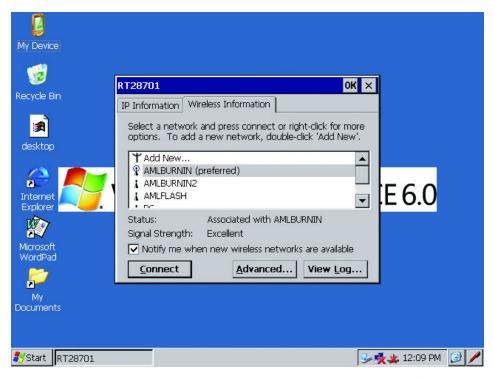
Once you are connected to a wireless network the Status will change and the Signal Strength will be displayed.
