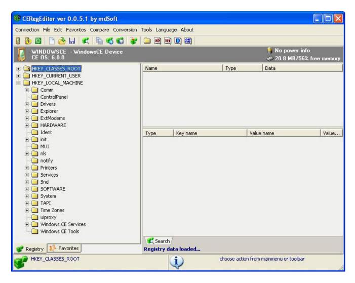
Connect the KDT900 to the PC via ActiveSync® and start the registry editor. To change the keys, edit the following registry keys as described:
