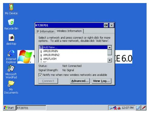
If the KDT900 has the optional Wireless radio, the unit will boot into the Windows Wireless setup menu. The unit will automatically search for available wireless networks.
