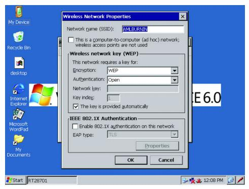
Many wireless networks require the proper passwords or network keys to connect. Contact your systems administrator to find out the proper network and password or keys.
