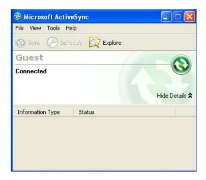
ActiveSync® will automatically create the connection and allow browsing from the PC to the device filesystem. Files can be copied to and from the KDT900 with Windows® Explorer.
