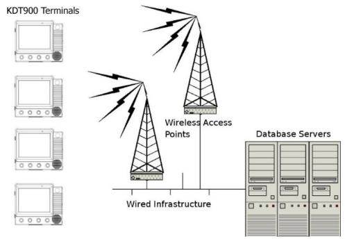
The range of the radio depends greatly on the quality of the Access Point and the RF communications characteristic of the environment where the device is used. The typical range for an 802.11 radio is 300 feet through free air. Additional Access Points must be added to improve coverage in a larger area, or in electrically noisy RF environments.
