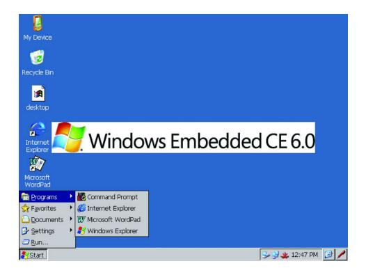
Tapping the touchscreen emulates a left mouse click in the desired area, and holding down a stylus or finger in one location will create a right mouse click.
