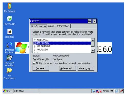
Use the KDT900 touch screen to select the wireless network you want to connect to. Note the unit is "Not Connected" under Status.
