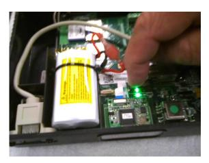
**4.** Make sure that the unit is powered on from an external power source (DC power or Power-over-Ethernet) for at least 12 hours before operating from the backup battery. If the backup battery has been fully drained from a power loss event, a charge cycle will take up to 24 hours.
