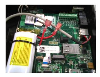
**3.** Release the safety switch and install the KDT750 or KDT900.
